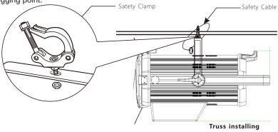
Regardless of the rigging option you choose for your PROFILE NF 200CW-MZ, always be sure to secure your fixture with a safety cable. The fixture provides a built-in rigging point for a safety cable on the hanging bracket as illustrated above. Be sure to only use the designated rigging point for the safety cable and never secure a safety cable to a carrying handle.
